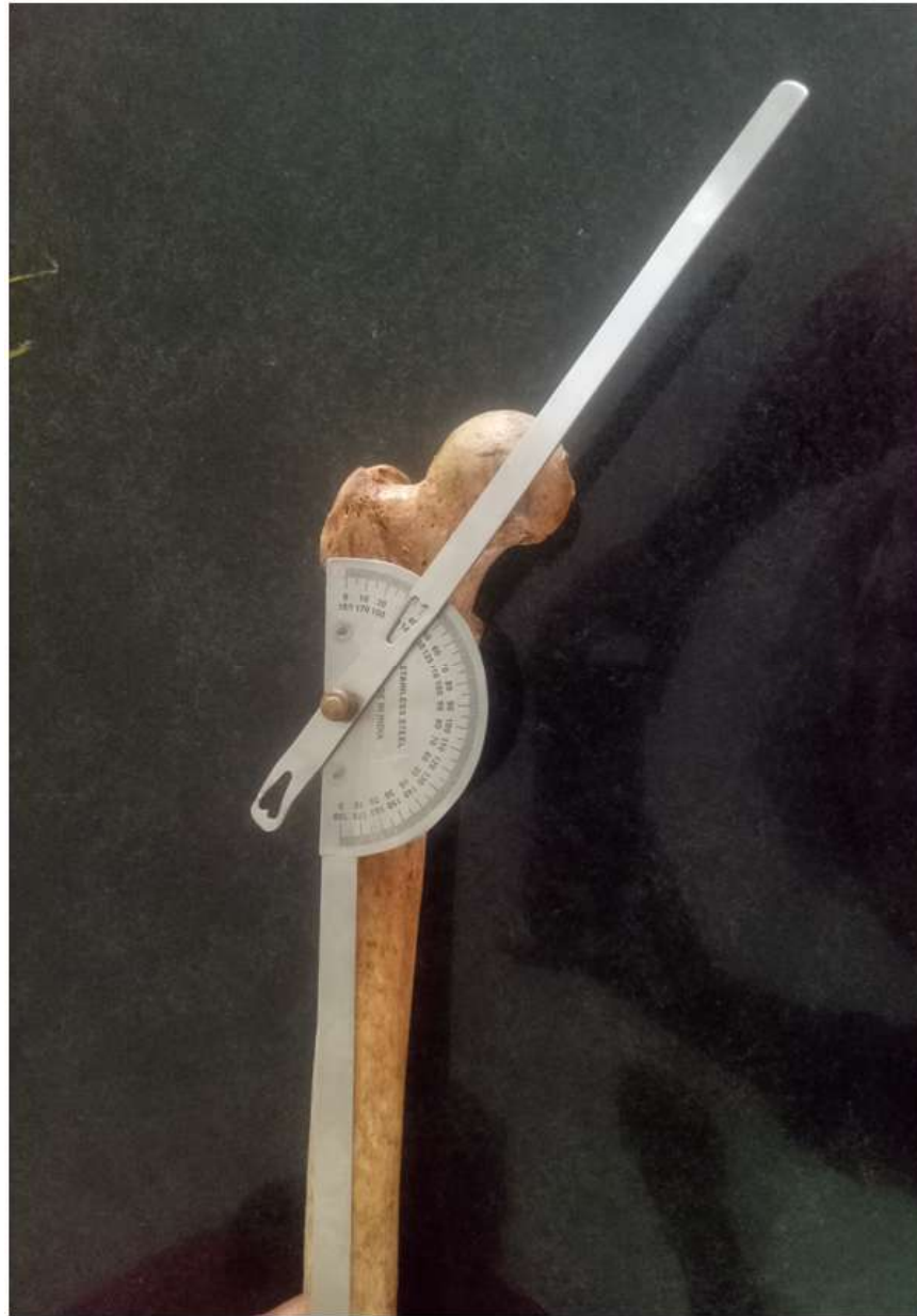
Fig. 1: Measurement of Femur Neck Shaft Angle using Goniometer
