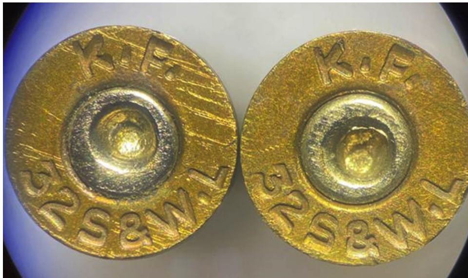
Fig. 1: Showing the Comparison of firing pin marks under Stereoscopic microscope, Created after firing over the percussion cap on 0.32 caliber cartridges.
