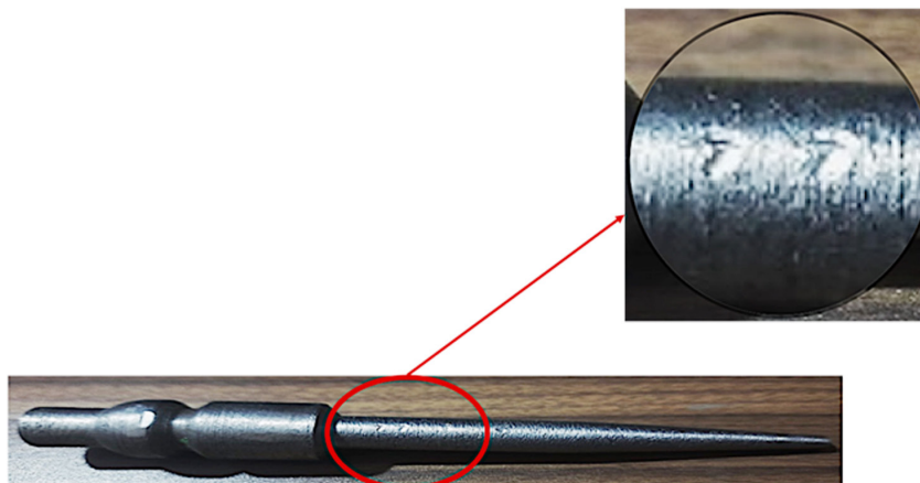
Fig. 2: Image of the specially designed firing pin engraved with micro-printed numbers with an enlarged view.
