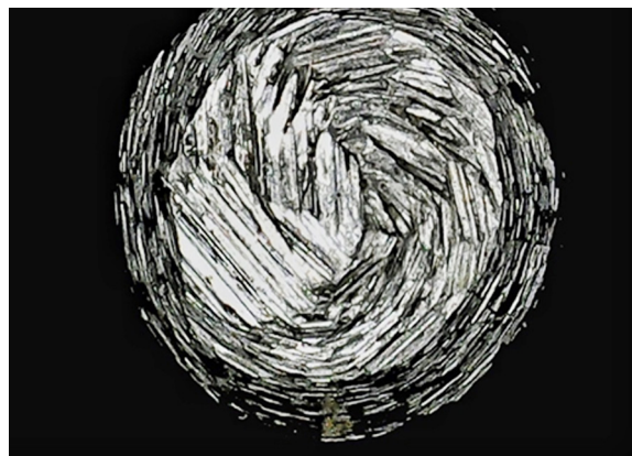
Fig. 3: The engraved markings at the tip of firing pin with the aid of Micro-Printing shown in magnified view under stereomicroscope.
