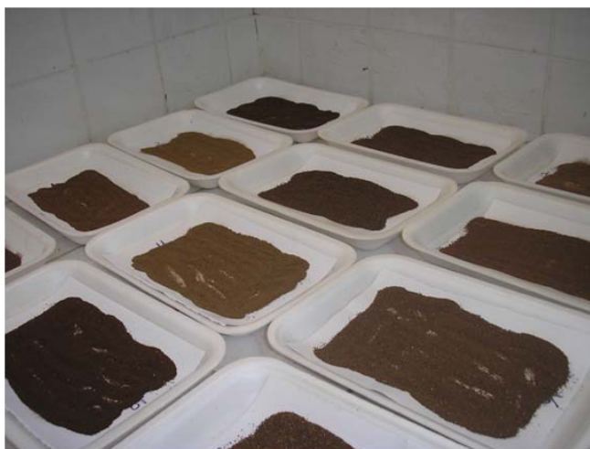
Fig. 3: A photograph of the soil samples drying in the laboratory.
