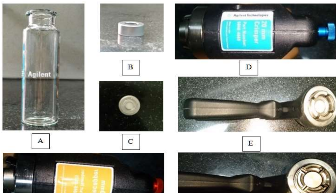
Fig. 10: Accessories of Gas Chromatography Headspace: A) 20ml GC-HS Vial, B) Metallic Crimp, C) PTFE Septa, D) Top View Crimper, E) Bottom view Crimper, F) Top View Decrimper, G) Bottom view Decrimper (Image source: Toxicology Lab, Deptt of FMT, AIIMS).
