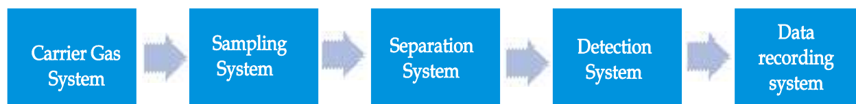
Fig. 4: Parts of a basic Chromatographic system.
